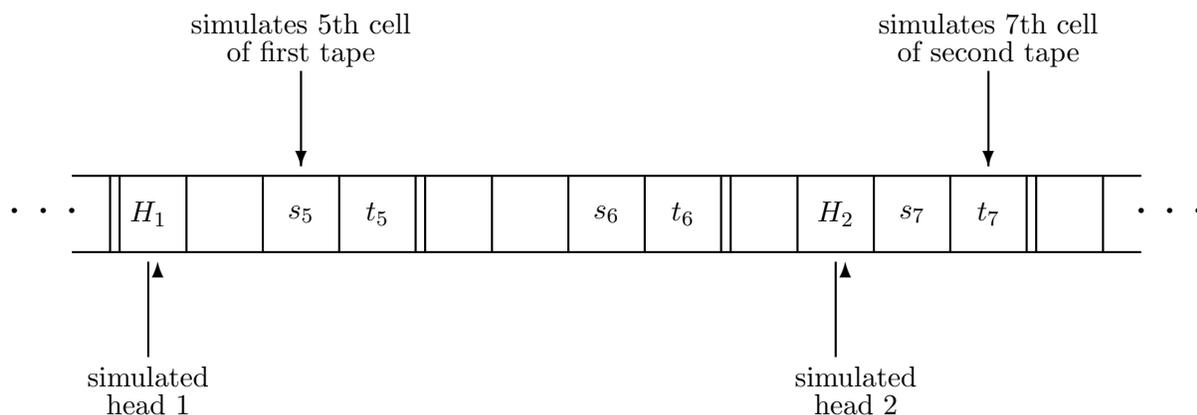
Figure 1.6: One tape simulating two tapes
