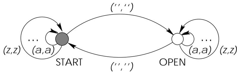
Figure 1.2: An automaton correcting quotation marks
