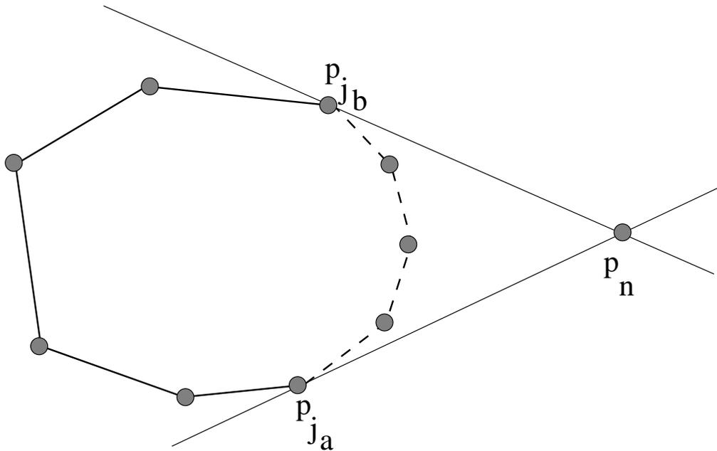
Figure 10.1: A simple convex hull algorithm
