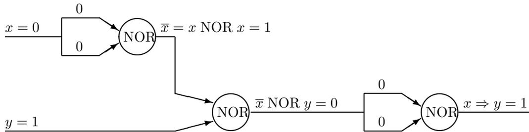
Figure 1.7: A NOR circuit computing  $x \Rightarrow y$ , with assignment on edges
